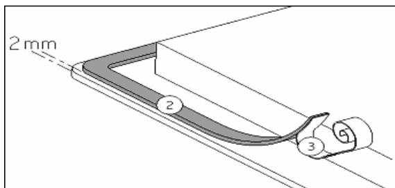
Stick the gasket (2) two millimeters from the external edge of the glass, after removing the protection tape (3).
